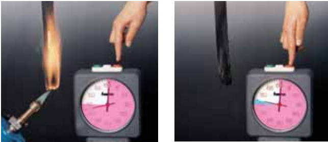
Flame-retardant belts cease to burn in seconds (green section) as soon as the gas flame is removed.
